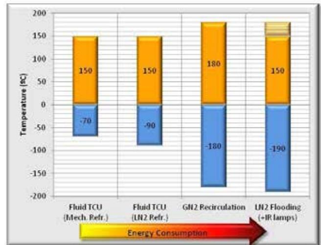
Standard ranges of applicability of the different thermal control technologies
